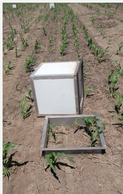
The new, larger gas chambers which will require less pruning of sorghum plants
